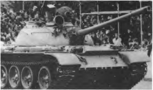
Figure 6-16. T-54/55 medium tanks. T-54 and T-55 tanks exist in numerous variations, all of which mount a 100-mm main gun and can be easily recognized by the large gap between the first and second roadwheels. The T-54A (above) mounts an AA machinegun in addition to coaxial and bow machineguns. The T-55 (below) lacks the AA machinegun.
